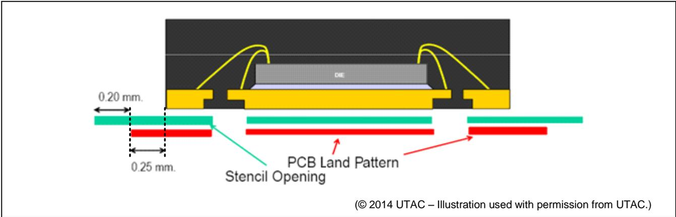
Figure 6.2 illustrates the recommended landing pattern for the ZSSC3018 QFN24 package.
