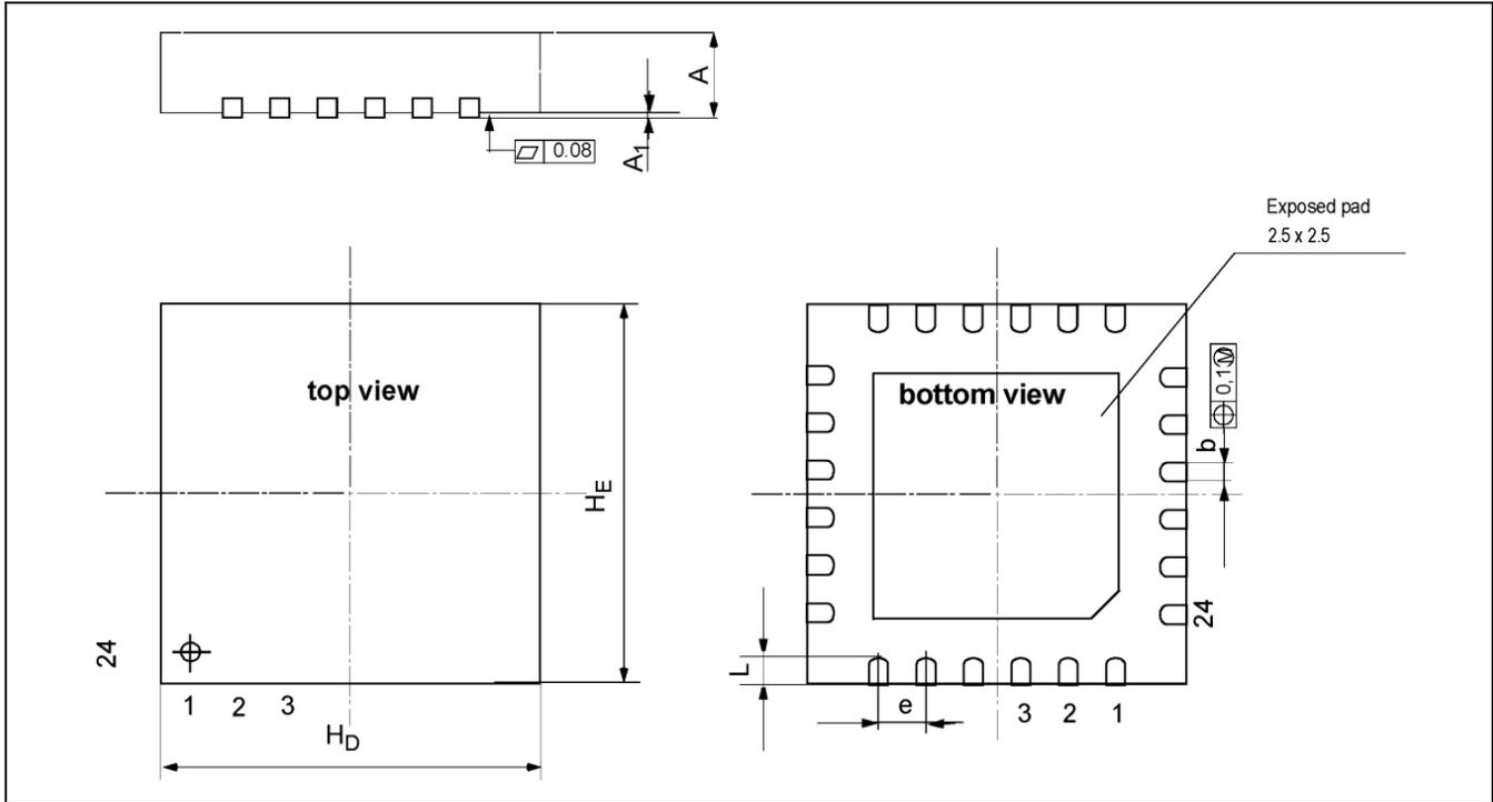
Table 5.1 QFN24 Dimensions (4mm x 4mm)
