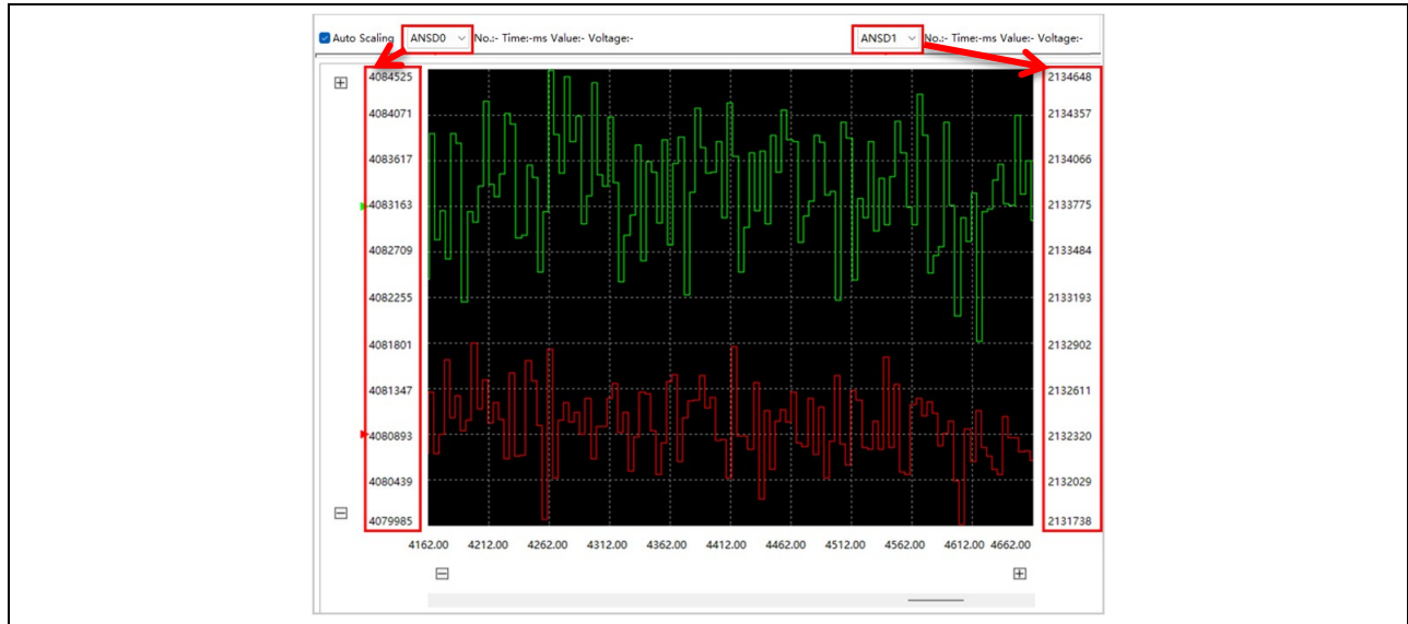
Figure 2 Waveform display screen in the "AFE Monitor (QE)" view: Waveform with vertical axis values
