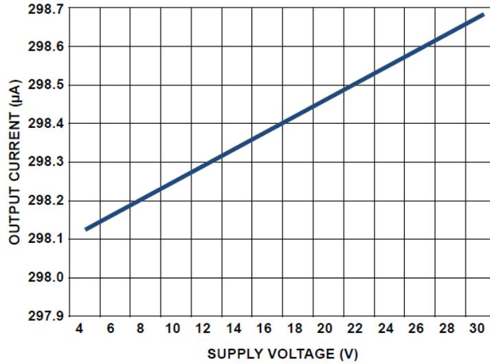
Figure 2. Output current immunity to supply voltage.
