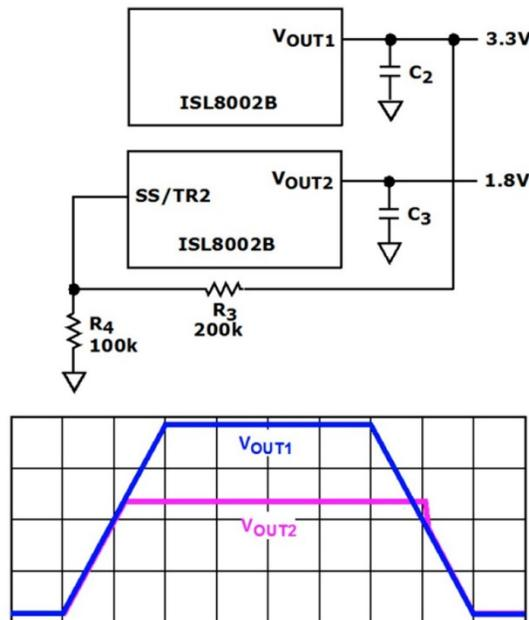
Figure 7. Coincidental tracking of  $V_{OUT1}$  to  $V_{OUT2}$
