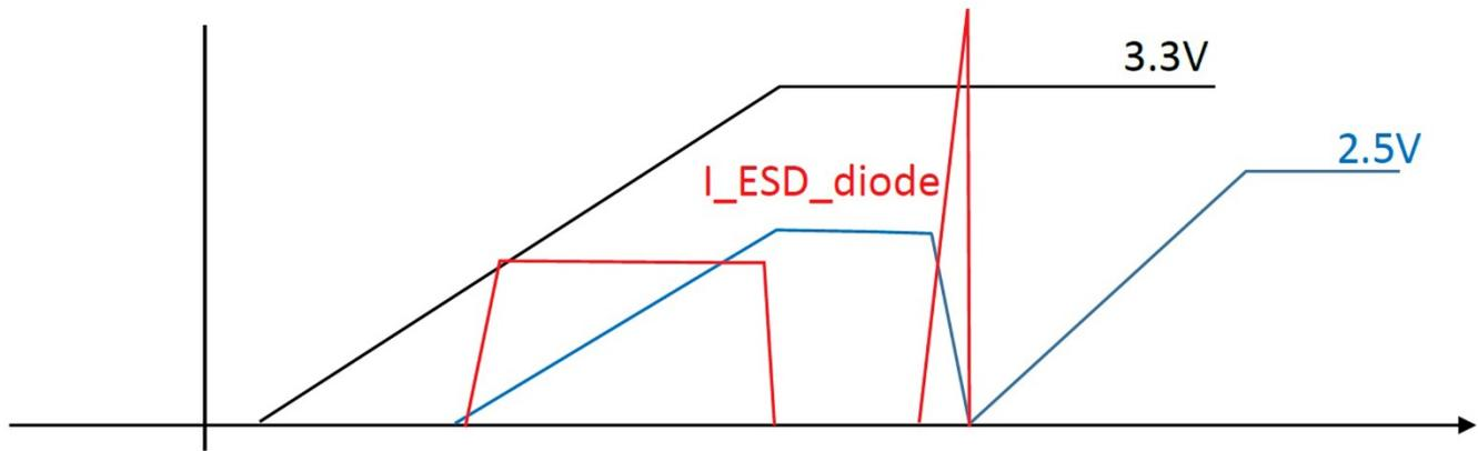
Figure 3. Startup waveform of 3.3V and 2.5V
