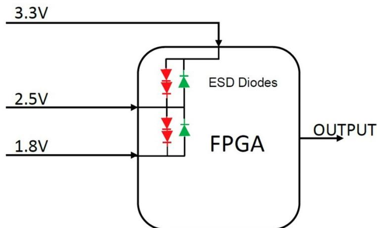
Figure 1. FPGA input block diagram
