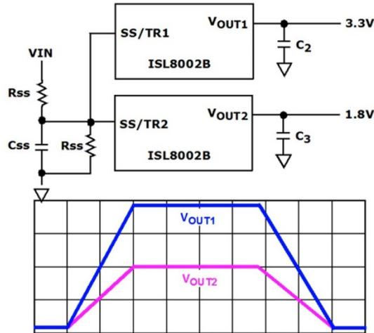
Figure 6. Ratiometric tracking of  $V_{OUT1}$  to  $V_{OUT2}$
