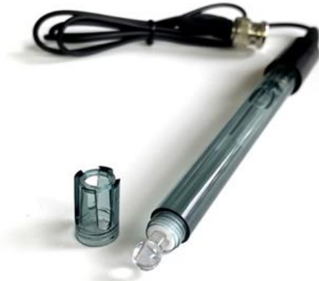
Figure 4: pH Electrode General View
