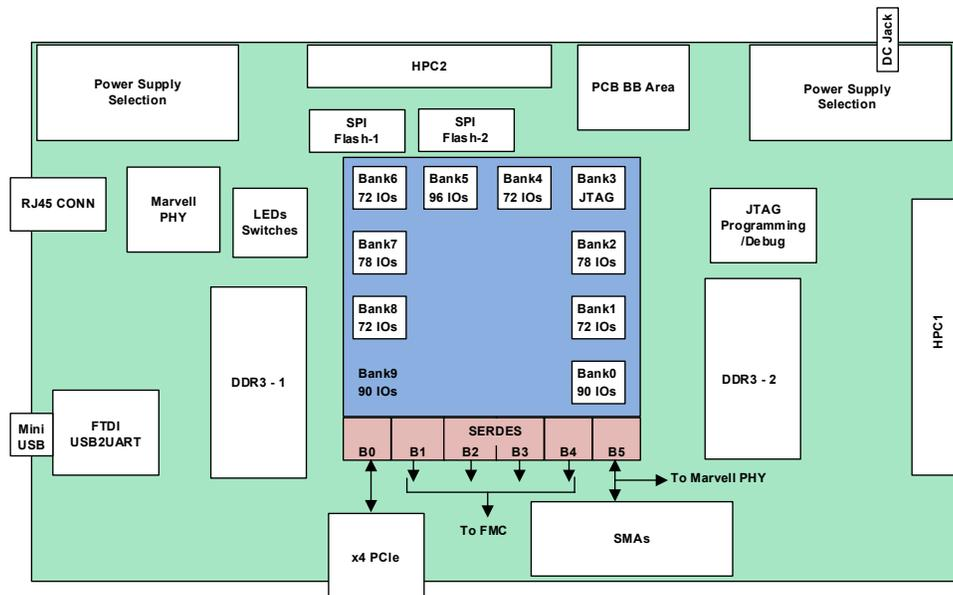
Figure 1. Block Diagram of the RTG4 Development Kit
