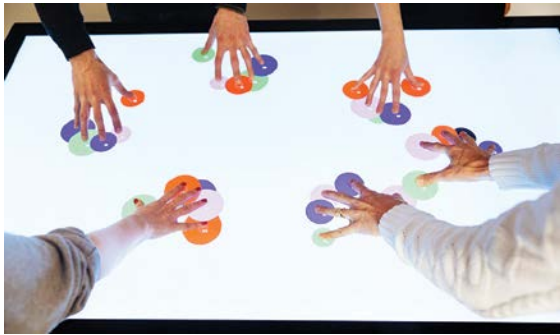
Figure 5: FlatFrog InGlassFORCE™ provides over 1000 pressure levels
