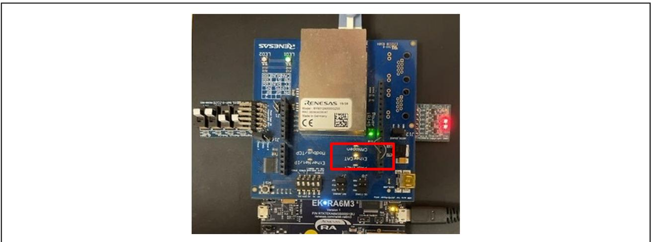
**Figure 3-43 Protocol LED: EtherCAT**
