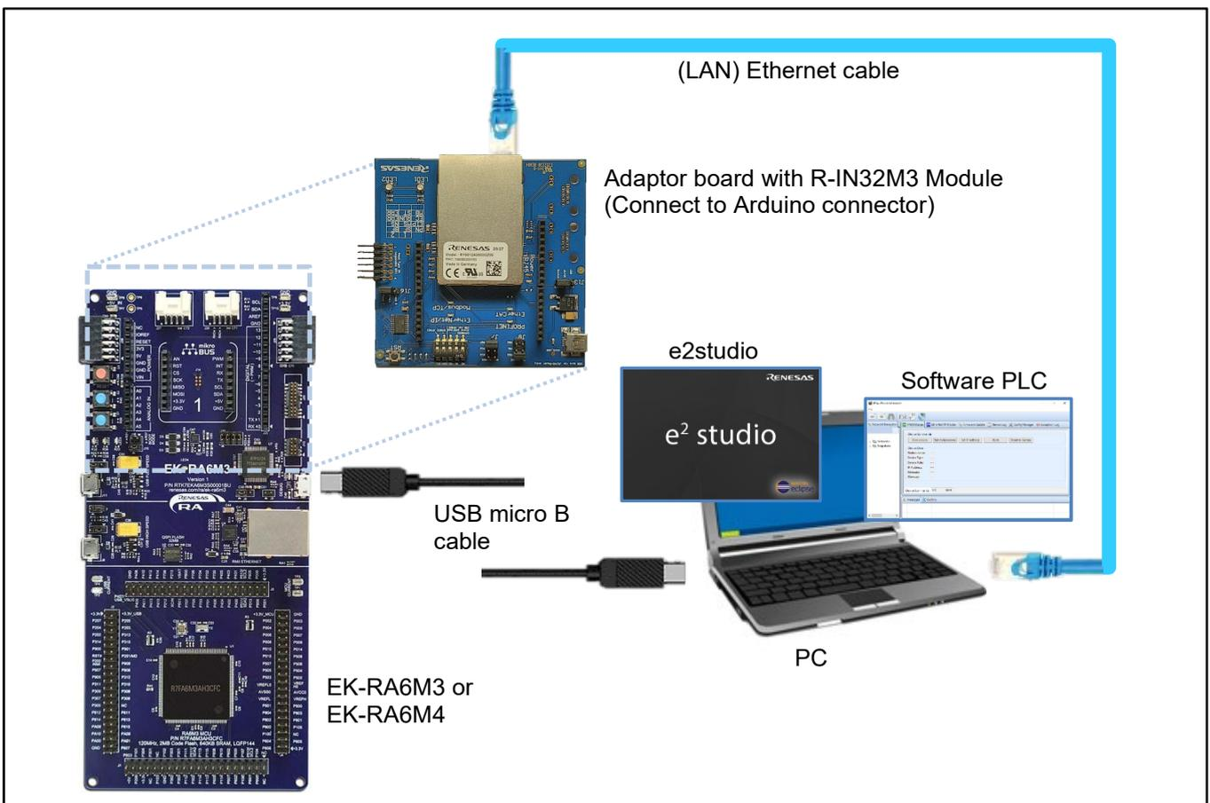
Figure 3-1 Connection configuration
