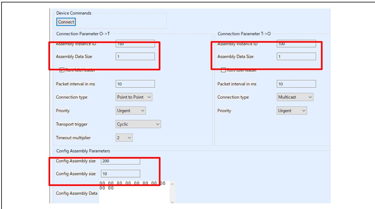
**Figure 3-38 Remote-IO application parameter**
