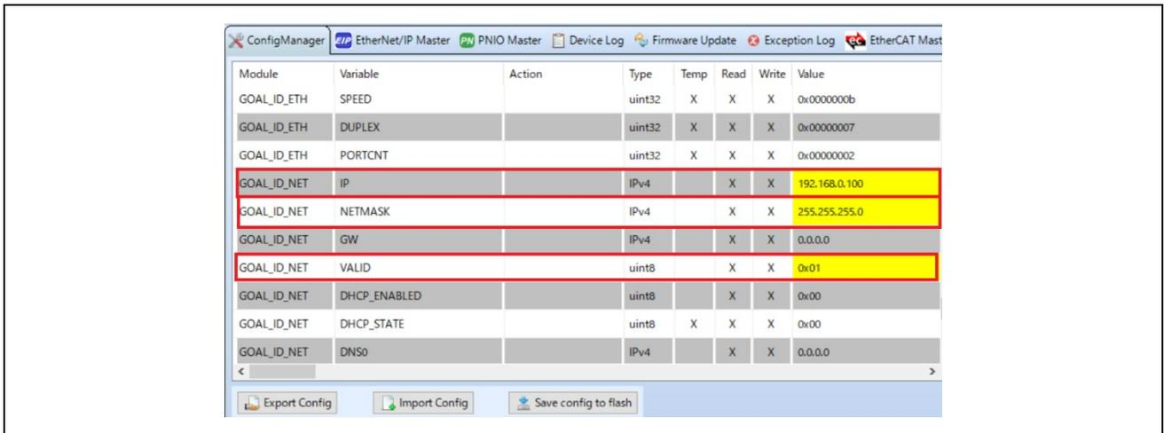
Figure 3-34 Set IP address on R-IN32M3 module
