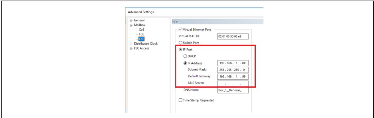
Figure 3.58 TwinCAT Network setting
