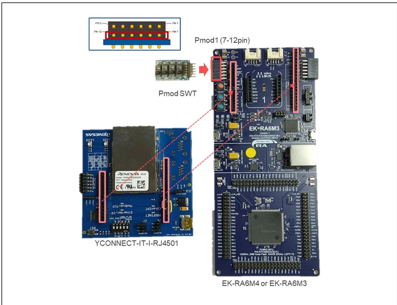
**Figure 2-3 Multi-protocol Selector Connection**
